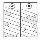
During installation, make sure that you mix the floor panels (and floor boxes) sufficiently so that there are not too many identical, lighter or darker planks next to each other. To obtain the best visual effect, it is best to install the panels in the direction of the longest wall and/or parallel to the incidence of light. And also install with the arrows on the underside all going the same direction.
