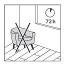
The glue must be able to cure 100% before moving in furniture. Hence, leave the floor untouched for 72 hours after installation between  $18-30^{\circ}$ C for the curing process to complete.
