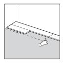
Draw a line along the first two dry fitted rows. This line marks to which point the glue should be applied.
